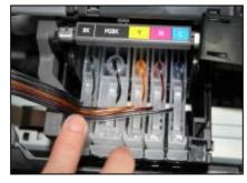
Then put the CISS cartridges into printer
